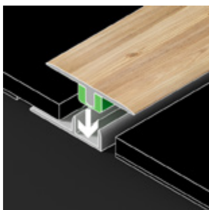
put the top profile in the base
