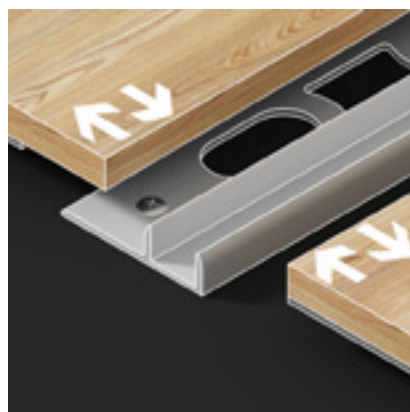
bring the floor boards close together, leaving enough space for expansion
