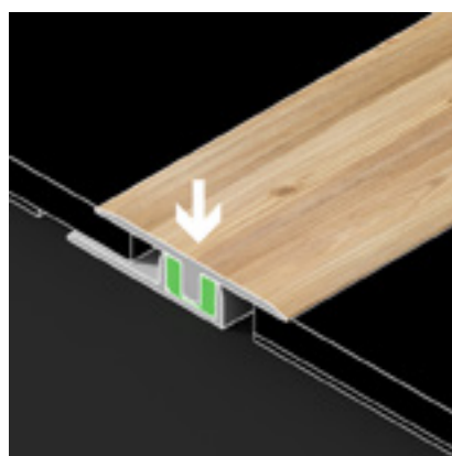
push the top profile in the base
